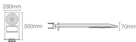
Features: • Katalyst™ Air Rain Shower • Cascade • Laminar flow • Ambient hydro-powered light
