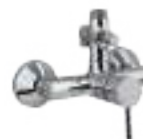
FLR-5145 Rs. 5,250 Single Lever Exposed Shower Mixer With Provision For Connection to Exposed Shower Pipe (SHA-1211NH or SHA-1213) & Hand Shower With Connecting Legs & Wall Flanges
